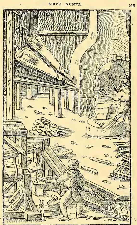
Reliquorū autē metallorū uenæ in fornacib. nō excoquūtur, sed argētū uti, ut eūā fabri, in ollis: plūbi cinerei, in canalibus. Sed primō dicā de argēto F 4. ΕΙΠΕ:
